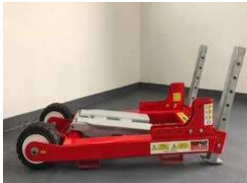
Trakjak's frame has two solid rubber wheels at the front, and two lower-link fixing brackets, with removable anchor pins, at the rear of the frame, to secure the tractor's linkage arms.
