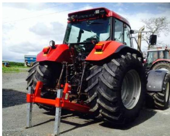
x. Lower the two support stands at the rear to the ground, and secure in the most suitable fixed position.
