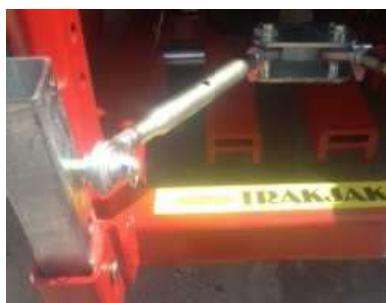
**When the connections are secure, the anchor pins can be withdrawn from the fixing brackets.**
