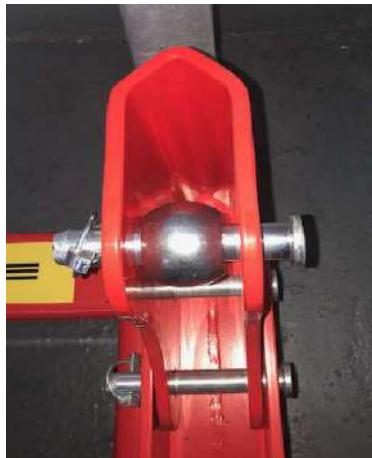
111. Fit the tractor's lower- linkage- ball to the lock pins, and reinstall.
